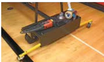
Storage trays with safety leg extenders
