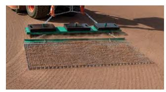
Add a steel mat drag for a cost-effective, one-pass solution.
