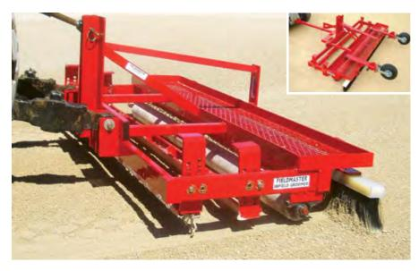
It's called the 'Fieldmaster Multi-Drag' for a reason. There's a lot going on. The spring scarifier tines help loosen infield soil, the dual leveling bar helps cut high spots and fill low spots. Then, a roller re-firms infield materials before a broom finishes the job. Rear tray allows weight to be added for better, more uniform soil penetration. Available with 3-pt hitch or tow-behind.
