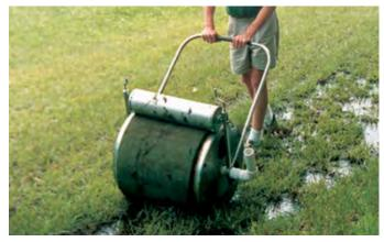
**Super Sopper** — Highly absorbent foam pad soaks up to  $\frac{3}{4}$ " of water with each pass. Top roller presses water into the holding tank which empties with a side drain elbow. Includes wheels for transporting and easy storage.
