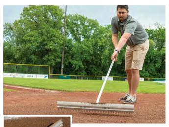
**Lute Scarifying Rake** — A leveling blade on one side and small tooth, small gap finishing blade on the other. The lute end is basically a straight edge that can be used for grading and leveling. The fine
