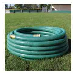
**GH Field Hose** — Handles working pressure up to 150 psi. PVC inner tube with a smooth cover of opaque green PVC compound reinforced with high-tensile yarn. *Lightweight and ozone / ultraviolet resistant.*
